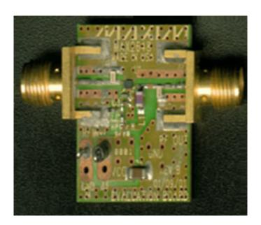
The MAX2648 is a high-linearity, silicon-germanium (SiGe) low-noise amplifier (LNA) designed for 5GHz wireless LAN systems based on 802.11a and HiperLAN2 standards. In order to achieve a low cost design, the device can be replicated using a FR4 type substrate with coplanar waveguide traces rather than the microstrip on Duroid used in the MAX2648 EV Kit.
